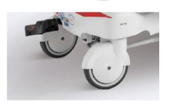
Four double-sided 6-inch casters, all lockable simultaneously using the foot pedal on both sides. TPR wheels resist wear even after 30 km of use. Features an antiwinding hard shell, integrated one-piece construction with no bolts.
